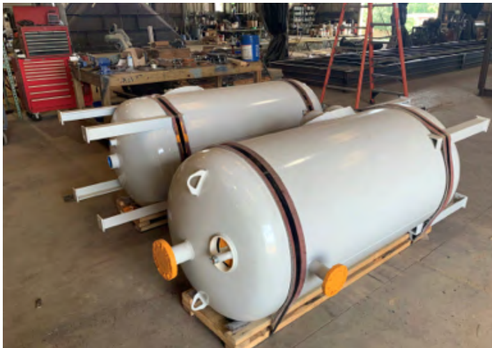
FABRICATION OF REGEN VESSELS
