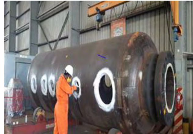
Magnetic Particle Inspection in progress
