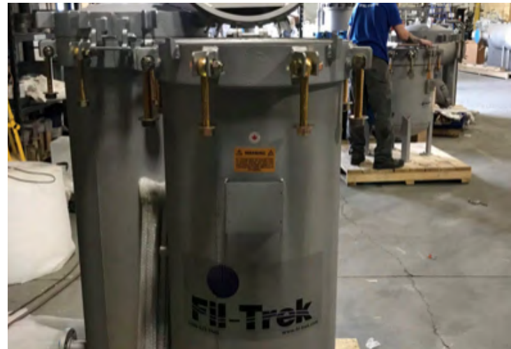
FABRICATION OF POLISHER VESSELS
